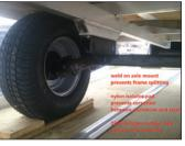
prevents frame cracking and our isolator pad prevents corrosion from dissimilar metals.
